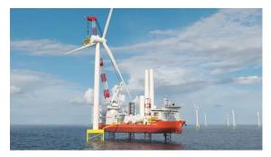
Figure 58 Turbine Installation Example with Jack Up Vessel
