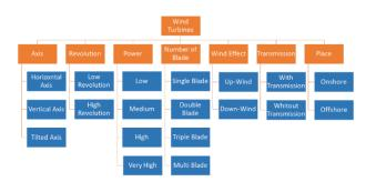
Figure 32 Wind Turbine Types
