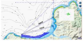
Figure 29 Fetch Distance from Installation Area to Coast According to Wind Direction
