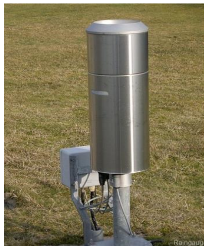
Figure 6: Self-recording or Automatic rain gauge (Pudyastuti, 2018)
