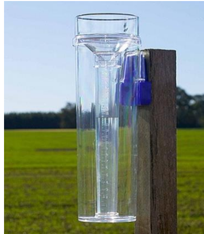
Figure 5: Ordinary or Non-automatic rain gauge (Pudyastuti, 2018)
